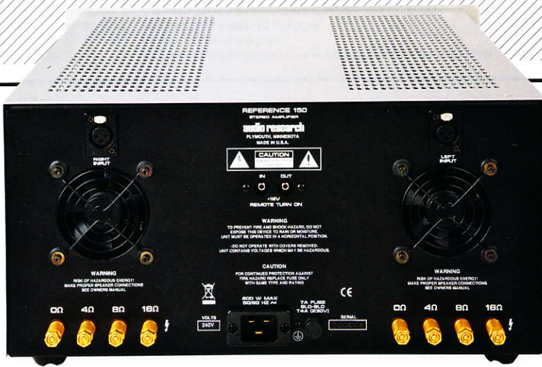
ABOVE: Balanced XLR inputs are joined by 4, 8 and 16ohm speaker connections (better suited to spades than 4mm plugs). Near-silent fans keep the interior cool
